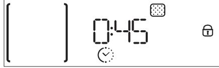
Once the cycle has been completed, the door remains locked until the temperature inside the oven has returned to a safe level.
